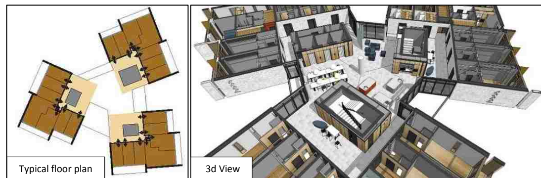
Figure 15: Accessibility pattern in the student housing of the University of Southern Denmark in Odense – Source: (“Student Housing / C.F. Møller”, 2016)
