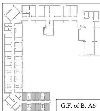
Figure 47: Location of bedrooms with ceiling light
